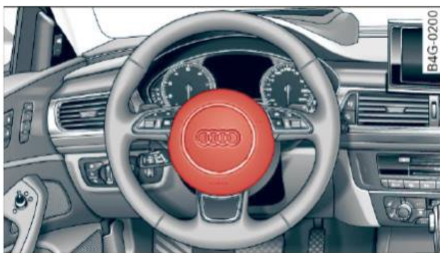
Fig. 156 Location of driver airbag: in steering wheel
