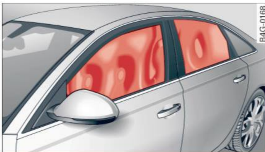
Fig. 165 Illustration of principle: Inflated side curtain airbags on the left side
