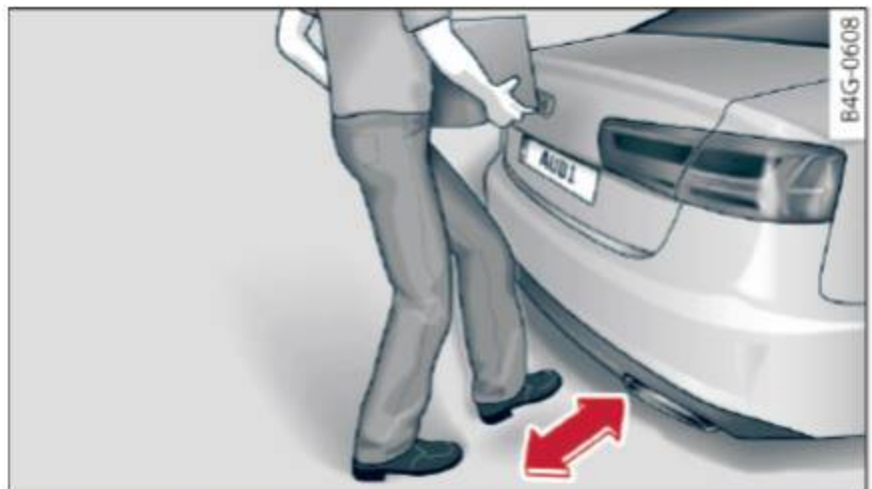
Fig. 30 Rear of the vehicle: foot movement
