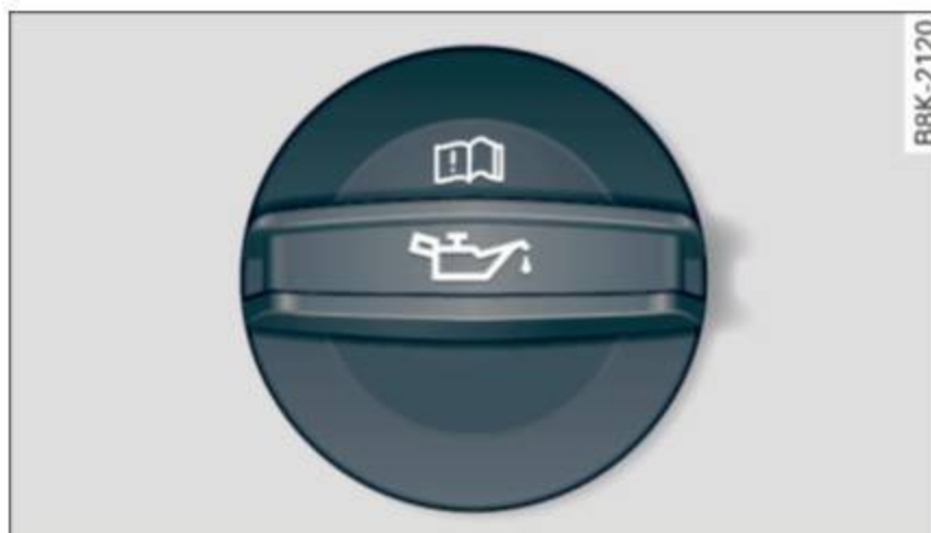
Fig. 188 Engine compartment: cover on the engine oil filler neck
