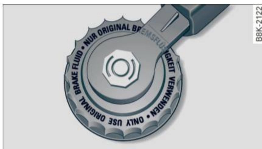
Fig. 190 Engine compartment: cover on the brake fluid reservoir
