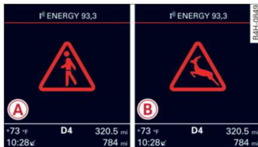
Fig. 112 Instrument cluster: (A) Pedestrian warning/(B) wild animal warning, when the image from the night vision assist is not selected in the instrument cluster display
