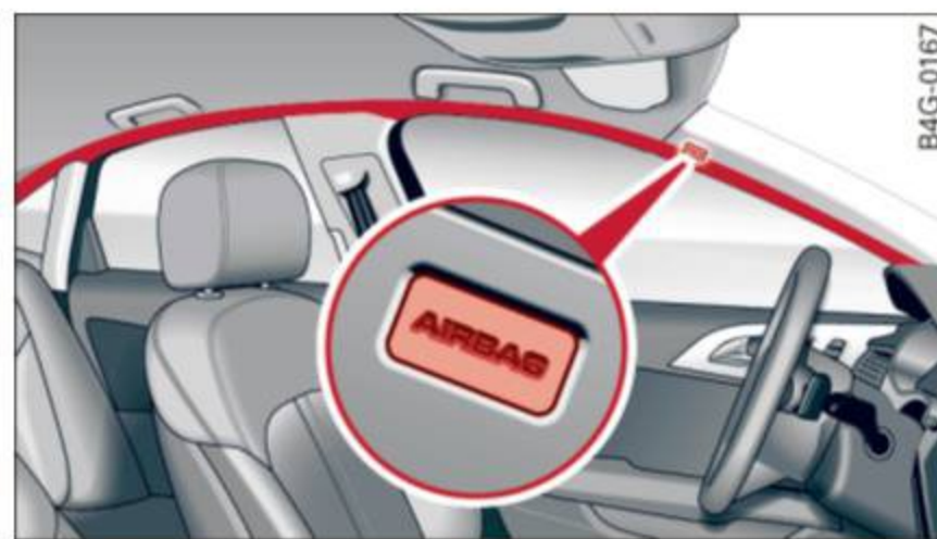
Fig. 164 Side curtain airbags, driver's side: side curtain airbag location
