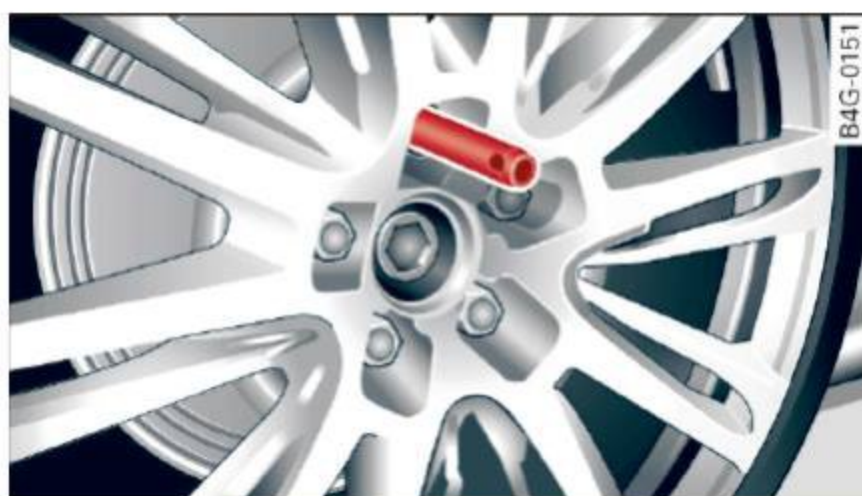
Fig. 209 Changing a wheel: alignment pin inside the top hole
