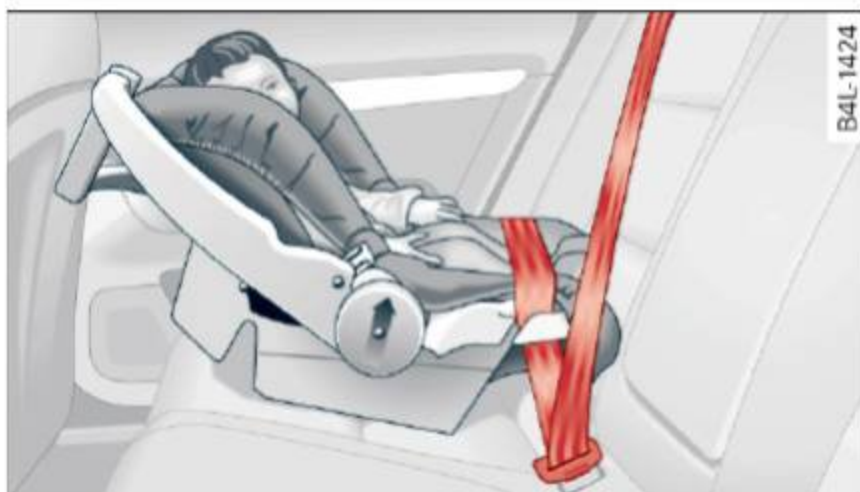
Fig. 167 Schematic overview: rearward-facing infant seat, properly installed on the rear seat
