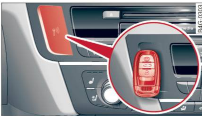
Fig. 81 Center console/master key: starting the engine when there is a malfunction
