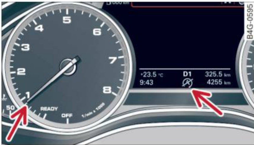
Fig. 84 Instrument cluster: Engine stop temporarily unavailable
