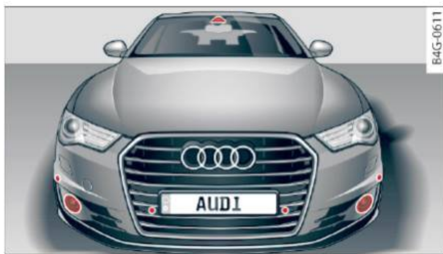
Fig. 88 Front of the vehicle: sensors and video camera
