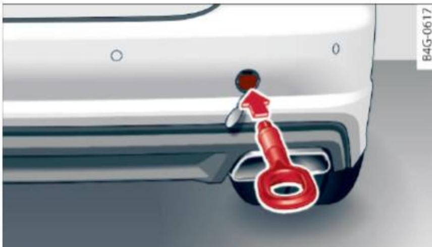
Fig. 219 Rear bumper: towing loop installed
