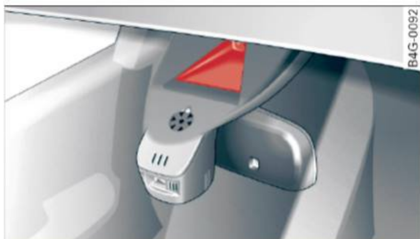
Fig. 100 Windshield: camera window for active lane assist
