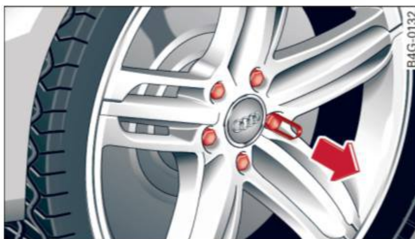
Fig. 203 Changing a wheel: removing the wheel bolt caps
