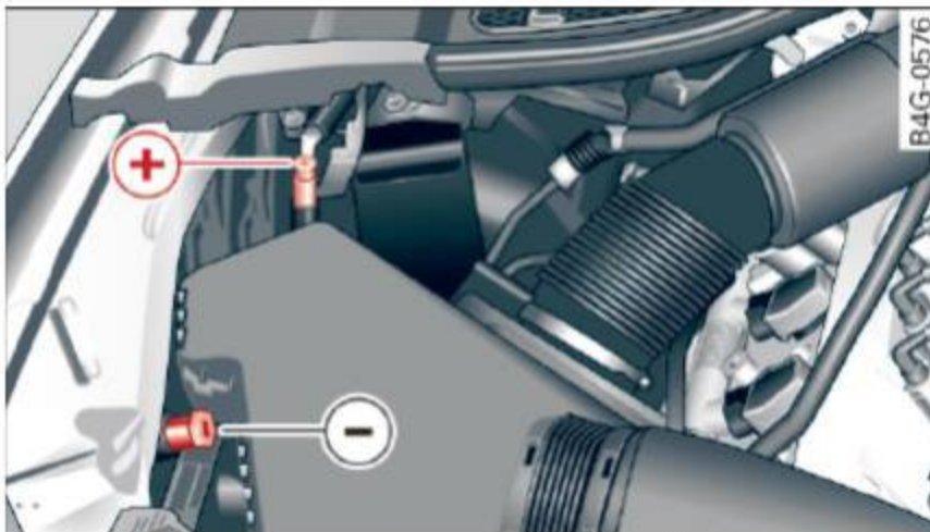
Fig. 214 Engine compartment: connectors for jump start cables and charger
