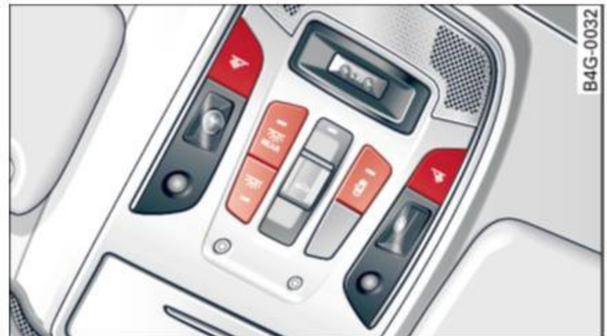
Fig. 42 Front headliner: interior lighting controls
