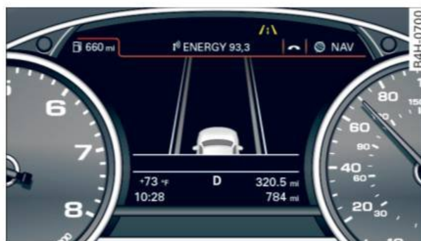
Fig. 102 Instrument cluster: active lane assist is switched on but not ready to provide warnings
