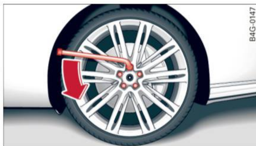
Fig. 204 Changing a wheel: loosening the wheel bolts
