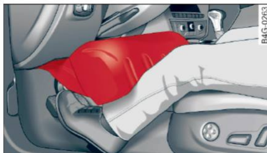
Fig. 161 Inflated airbags protecting in a frontal collision
