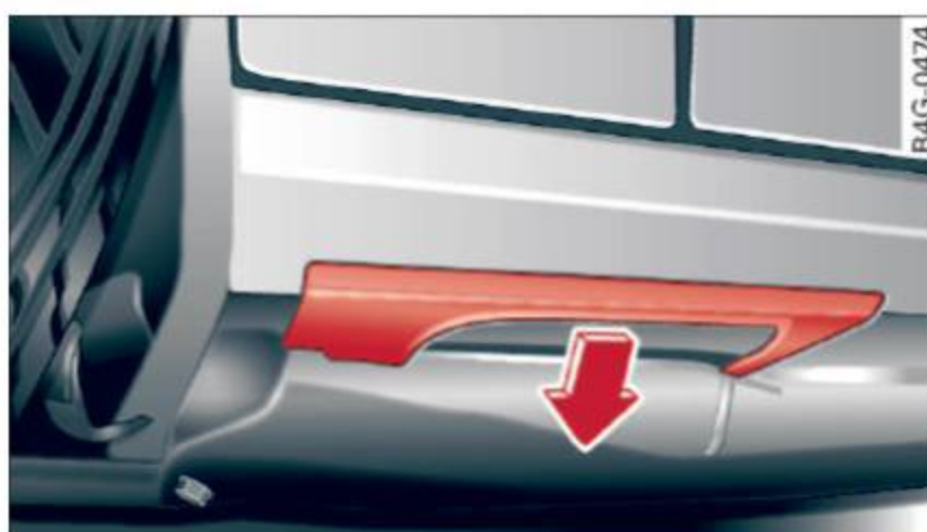
Fig. 207 Sill: removing the cover
