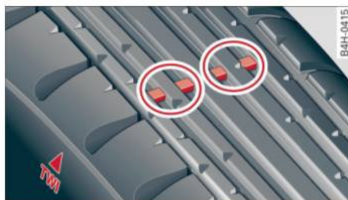
Fig. 194 Tire profile: Treadwear indicator
