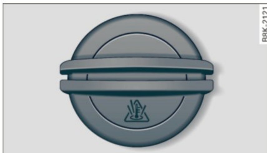
Fig. 189 Engine compartment: cover on the coolant expansion tank
