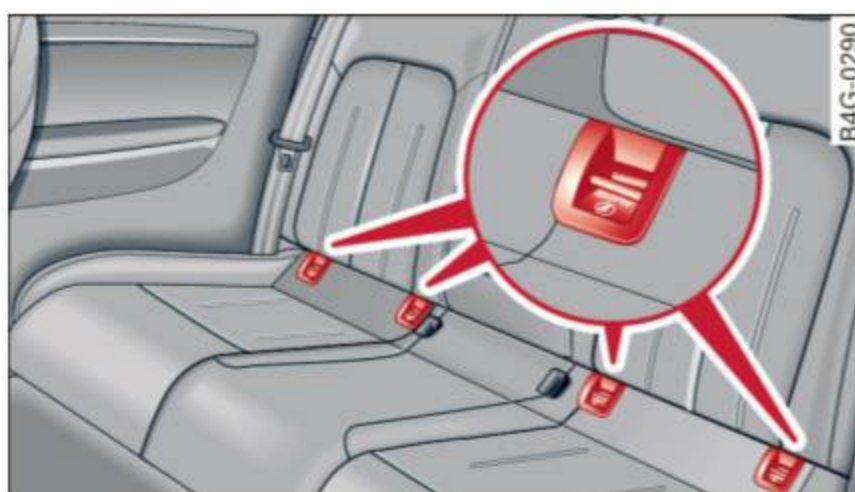
Fig. 173 Rear seats: lower anchorage bracket locations
