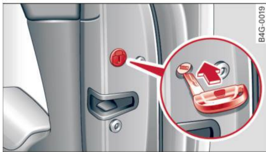
Fig. 25 Door: Emergency locking
