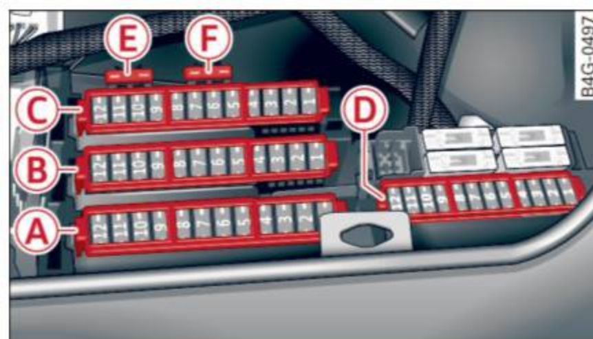
Fig. 213 Luggage compartment: fuse panel with plastic clip
