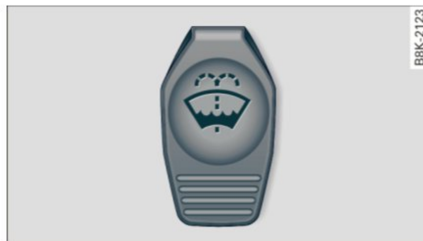
Fig. 192 Engine compartment: cover on the windshield and headlight* washer fluid reservoir
