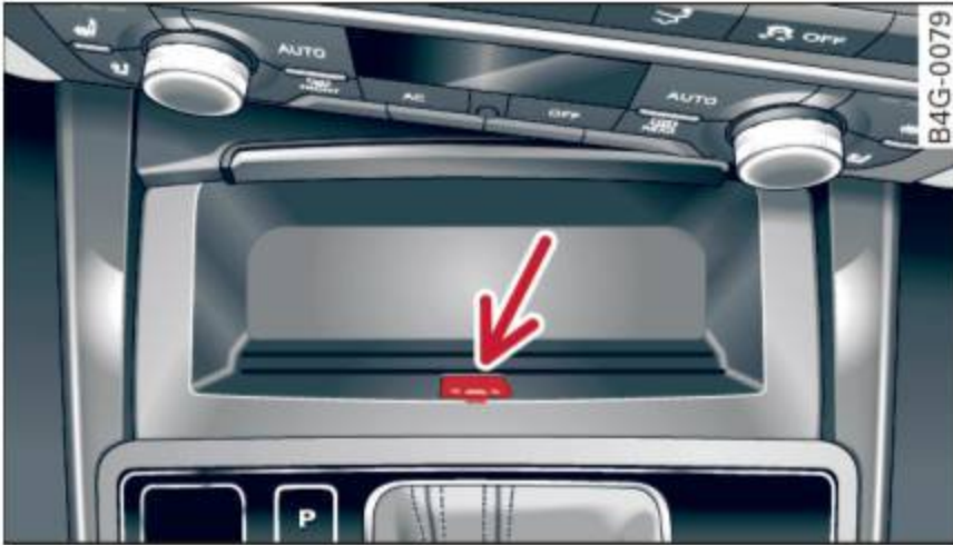
Fig. 119 Front center console: Selector lever emergency release
