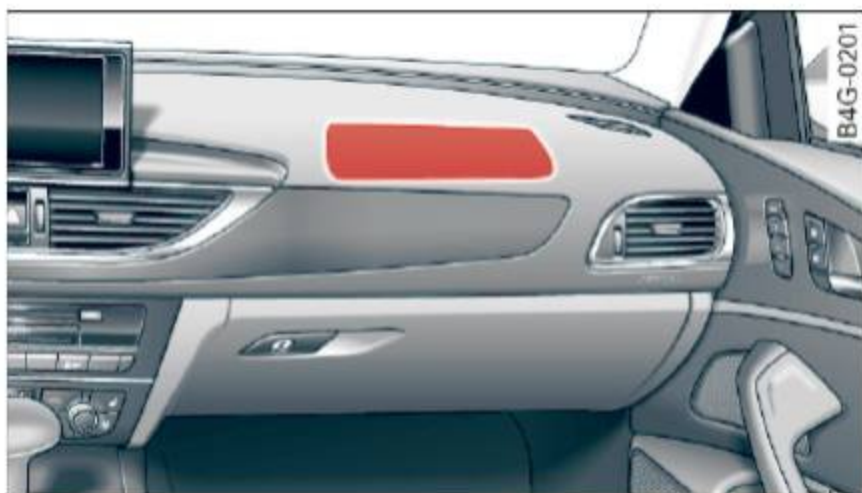
Fig. 157 Location of front passenger's airbag: in the instrument panel
