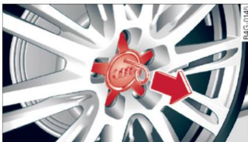
Fig. 202 Changing a wheel: Removing the wheel cover
